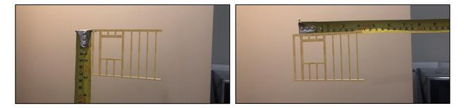
*Note.* Research participant C provided these two photographs. They show a physical tape measure measuring the dimensions of a scaled virtual 3D wood panel model projected to an interior space by 3D Warehouse®. The left picture shows the tape measure measuring the overall height of the virtual wood stud wall model, and the right picture shows the tape measure measure measure measure the width of the window opening. The link to larger JPG versions is:
