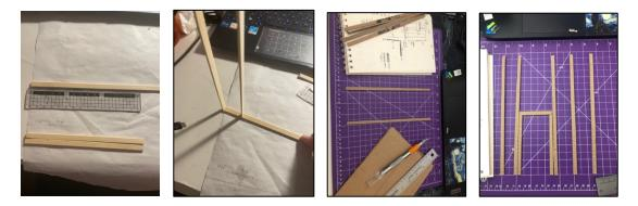
*Note.* Two research participants provided these four screen captures. Two pictures on the left show the physical model being constructed using balsa wood strips, and two pictures on the right show it being constructed using cardboard strips. The link to larger JPG versions is: https://www.notion.so/Dissertation-Yi-Lu-Figure-22-182408515282807fa0e1f49bf6e16bbd
