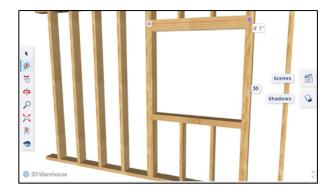
*Note.* Research participant D provided this screen capture. It shows that the measuring tool in SketchUp® measures the width of the window opening of a 3D model. The link to a larger JPG version is: <u>https://www.notion.so/Dissertation-Yi-Lu-Figure-16-</u>
