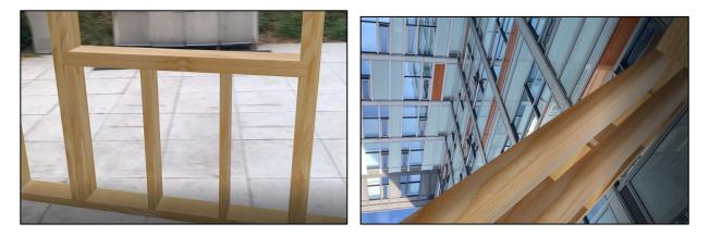
*Note.* Research participant D provided these two screen captures. The left picture shows the model rendered with wood grain textures, making it easier to identify how various wood members were connected and constructed. The picture on the right shows the arrangement of wood lintels in the opening and how other wood studs supported the top plates. The link to larger JPG versions is: <u>https://www.notion.so/Dissertation-Yi-Lu-Figure-13-</u>
