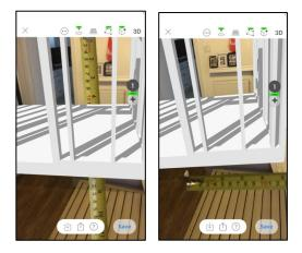
*Note.* Research participant E provided these two screen captures. They show a physical tape measure measuring the dimensions of a scaled virtual 3D wood structure model projected to an interior space by ARki®. The picture on the left shows the thickness of the bottom wood platform, and the picture on the right shows the width between two wood studs. The link to larger JPG versions is: <u>https://www.notion.so/Dissertation-Yi-Lu-Figure-21-</u>
