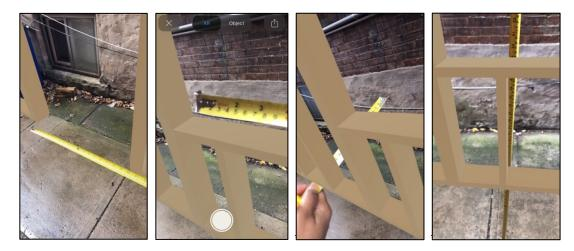
*Note.* Research participant E provided these four screen captures, showing a physical tape measure measuring the dimensions of a true-size virtual 3D wood panel model in 3D Warehouse®. The picture on the left shows the measurement of the door opening width. The second picture from the left shows the width of the window opening. The second picture from
